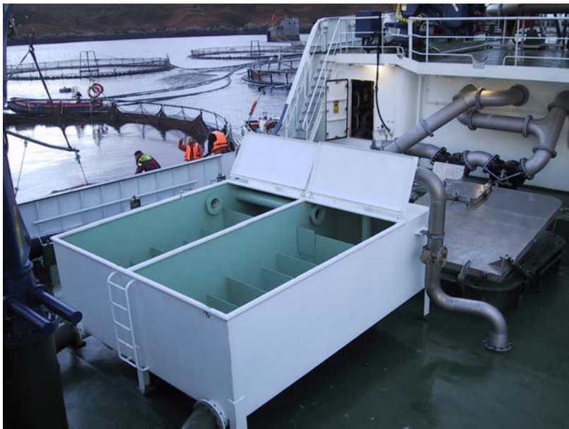
Figure 12. Water treatment unit (degasser) on one well boat designed for closed transport. Photo: Kai Sørensen (NIVA)
