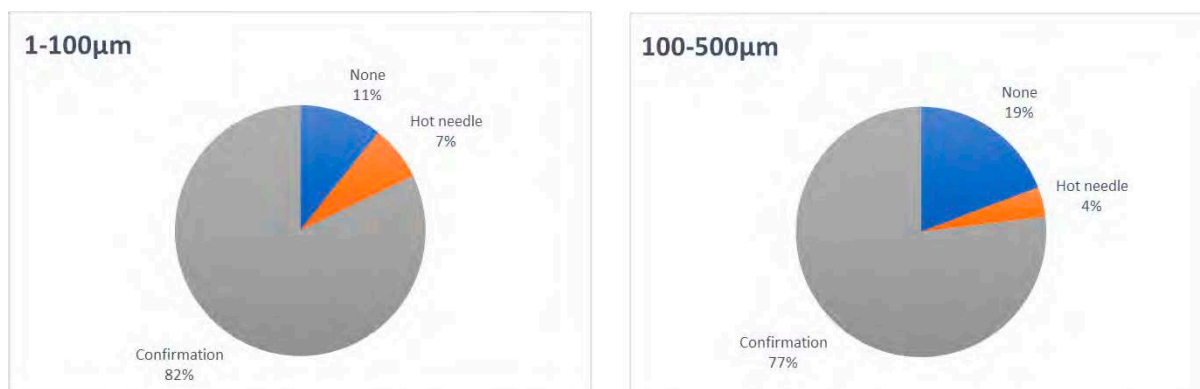
Figure 3.1.3-3 Use of confirmatory techniques when working with microplastics. The citatory confirmation includes both Raman and FTIR analysis on all or a subsample of microplastics.
